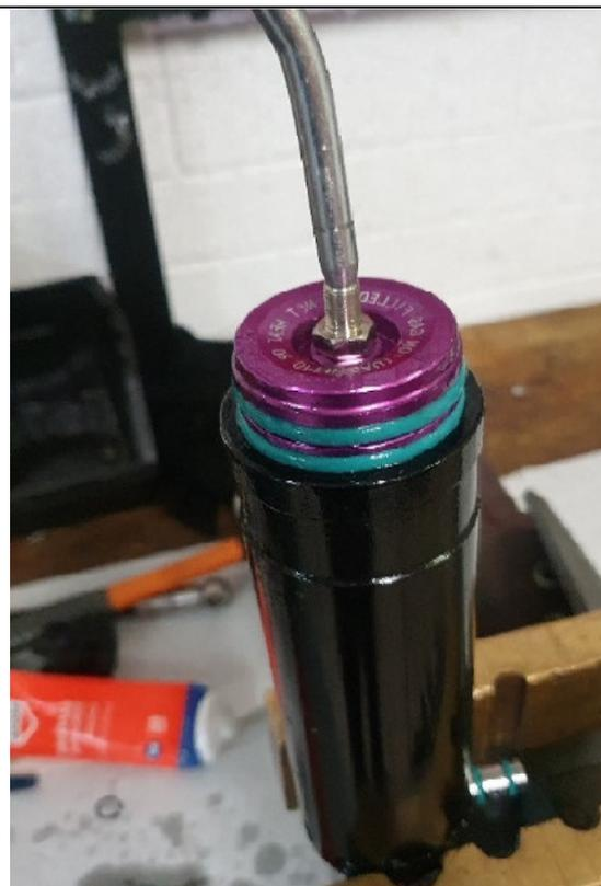
17. Regrease the circlip groove and remove the floating piston with a puller tool (22 x 1.5mm thread). Change seals or wear bands if required - inspect D-Ring to ensure it is not damaged.
