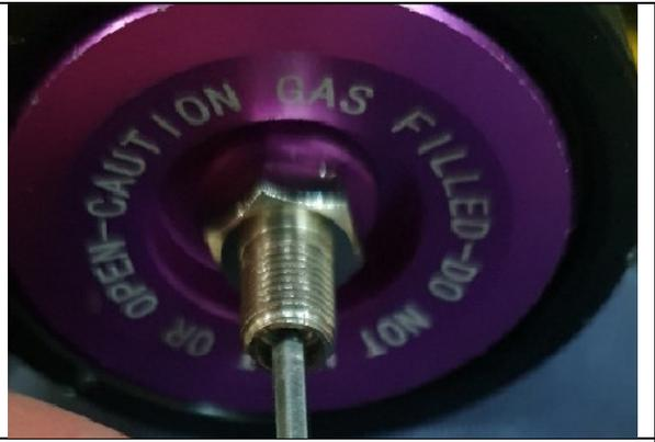
4. Push down seal head assembly. This is often very tight and may require a cut tube spacer between the rod end and seal head assembly while you use a rubber mallet to hammer down the rod end to push down the seal head assembly.
