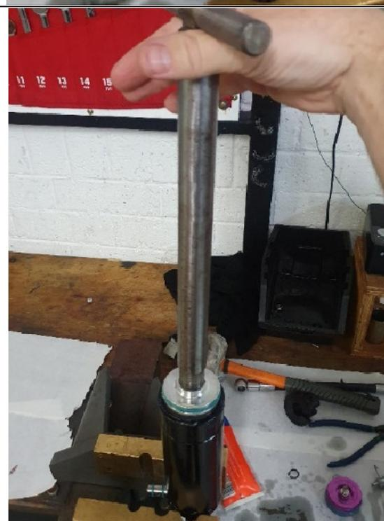
18. Change hose or hose fittings as required – use circlip pliers to remove the circlip, pop off the hose. Change the o-rings (the larger inside diameter O ring goes against the body/res and the smaller to the outside. Grease up and refit hose and circlip ensuring circlip is seated.
