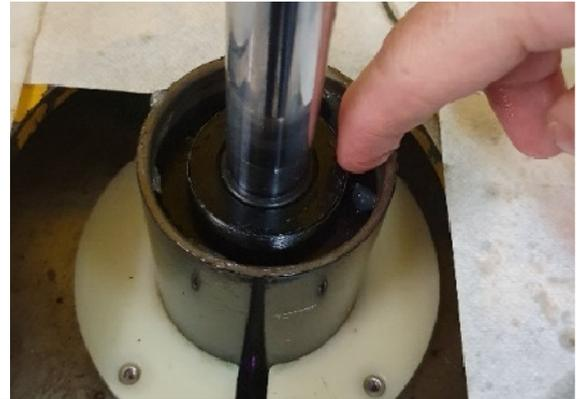
7. Pull up the rod and seal head assembly together, wriggling as you go and remove from shock. This can also be quite difficult and may require you to pull it up, push it back down, regrease the circlip groove and try again or hold the rod end and shaft in softjaws vice while you tap the body down with a rubber mallet.
