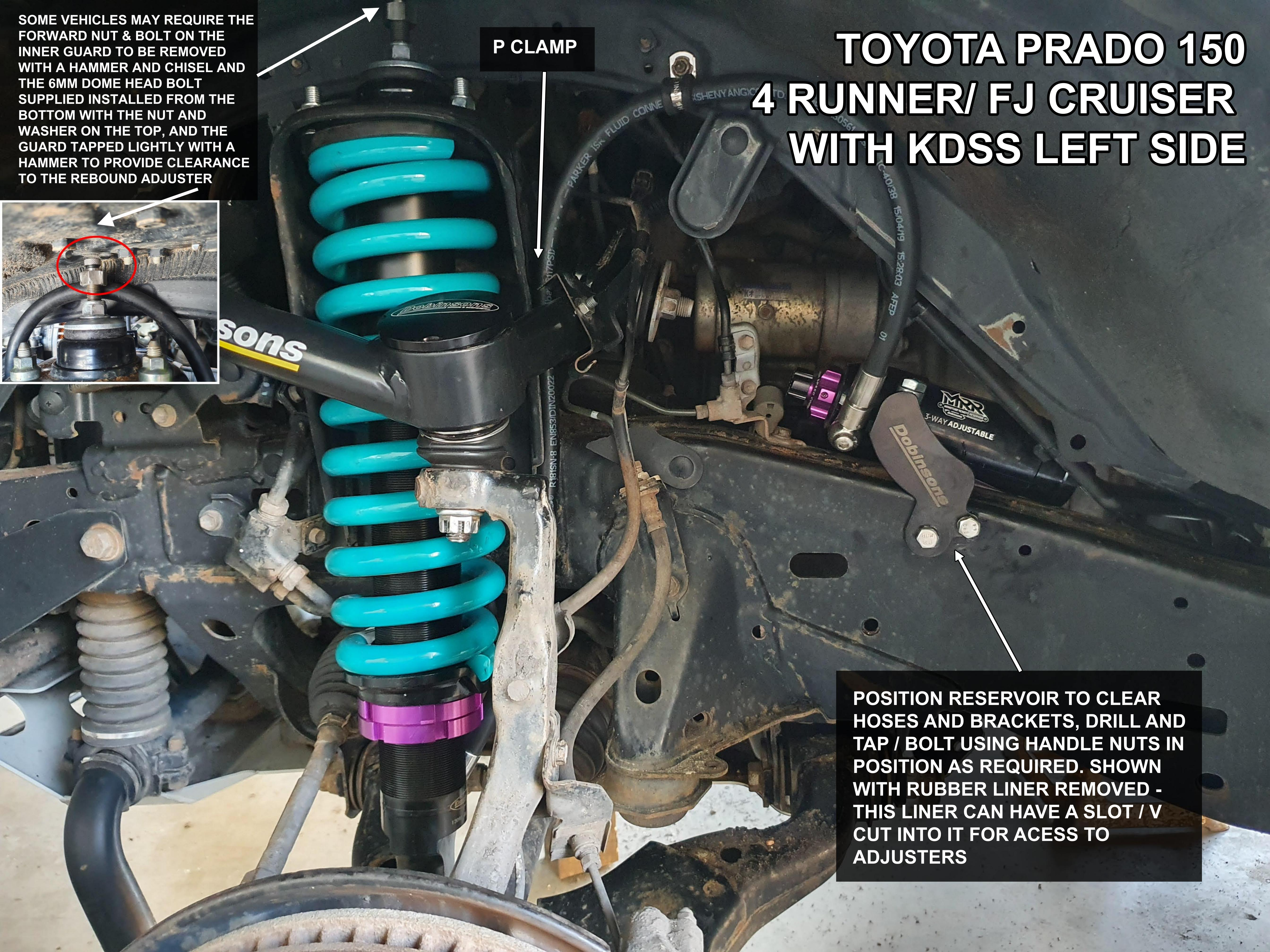
SOME VEHICLES MAY REQUIRE THE FORWARD NUT & BOLT ON THE INNER GUARD TO BE REMOVED WITH A HAMMER AND CHISEL AND THE 6MM DOME HEAD BOLT SUPPLIED INSTALLED FROM THE BOTTOM WITH THE NUT AND WASHER ON THE TOP, AND THE GUARD TAPPED LIGHTLY WITH A HAMMER TO PROVIDE CLEARANCE TO THE REBOUND ADJUSTER
