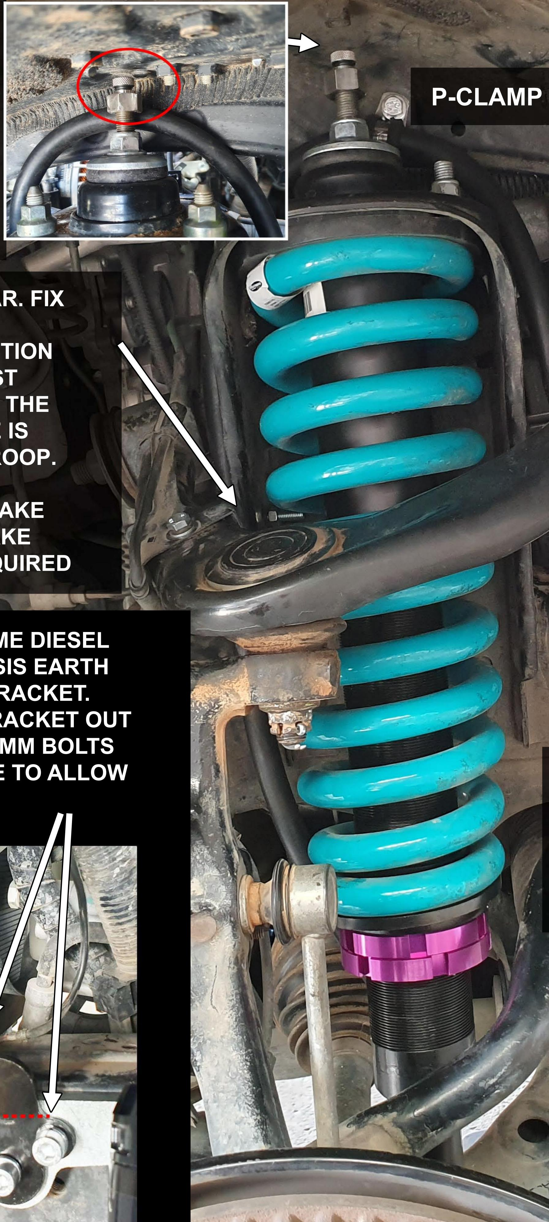
**ROUTE HOUSE TO THE REAR. FIX** HOSE WITH P - CLAMP. **DRILL 6MM HOLE AND POSITION** CLAMP SO HOSE IS AGAINST THE OUTER FOLD EDGE OF THE **COIL TOWER AND SO HOSE IS** ALMOST TIGHT AT FULL DROOP.
