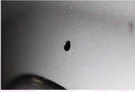
Using a 114mm hole saw or similar carefully drill the 2 snorkel body inlet holes on low speed.
