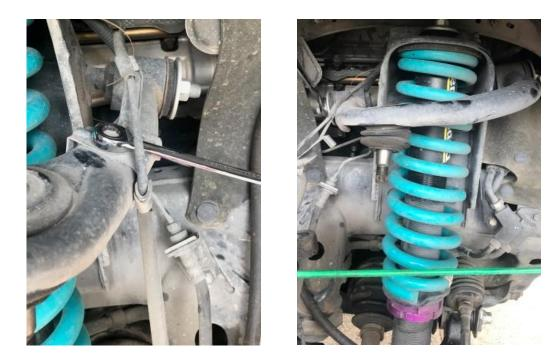
3. Using OE bolts and supplied bush washers loosely bolt the Dobinsons UCA into the OE chassis mounts, using the Left and Right arms. Fit the supplied washers to the outside of the arms (outsides of either end bushes). This should look like the OE fitment.
