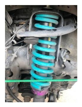
3. Using OE bolts and supplied bush washers loosely bolt the Dobinsons UCA into the OE chassis mounts, using the Left and Right arms. Fit the supplied washers to the outside of the arms (outsides of either end bushes). This should look like the OE fitment.
