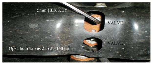
iv. Once spring installation complete vehicle must be placed on level ground before turning KDSS valves to a closed position (turn in a clockwise direction to achieve this.)
