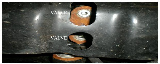
iii. Insert a 5mm hex key into one recess at a time and turn both valves 2 to 2.5 full rotations in an anti clockwise direction. (The KDSS is now disengaged and sway bar ends should be freed and manipulated with little effort.)
