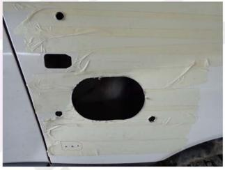
13. Using the step drill, drill a few larger holes in the centre of the new indicator position. This will allow you to start to cut the shape out with the pneumatic hacksaw.
