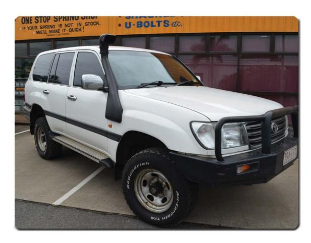
This Snorkel will take approximately 2 hours to install and is installed to the Right Hand Side of the vehicle.
