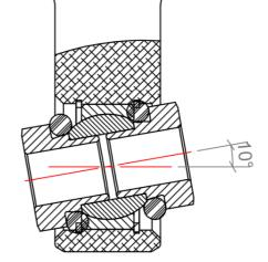
HIGH ANGULAR TRAVEL APPLICATIONS -O-RINGS REMOVED, HI-ANGLE SPACERS FITTED. MAX APPROX. 19°
