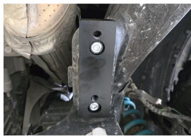
4. When reinstalling the OE sway bar onto the relocation brackets it is important to support the OE bracket with a screw jack and ensure the holes line up and is sitting flat against the relocation bracket.
