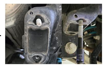
3. Install the sway bar relocation brackets with the threaded holes toward the front of the vehicle using the supplied alen head bolts.
