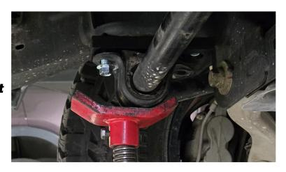
4. Reinstall the sway bar onto the relocation bracket using the supplied bolts.
