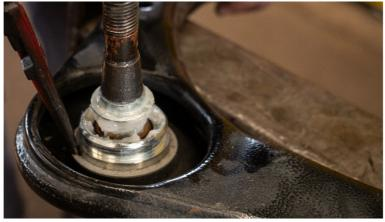
3. Use press tools as shown below. DO NOT PRESS ON THE END OF THE THREAD UNDER ANY CIRCUMSTANCES. Ensuring you press from the housing to prevent damage.
