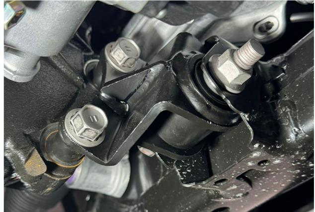
Install the passenger-side mount, reusing the OEM hardware and the two supplied M16 nuts.
